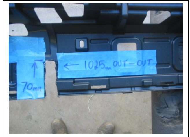
Figure 14 – Cut end of grille.
