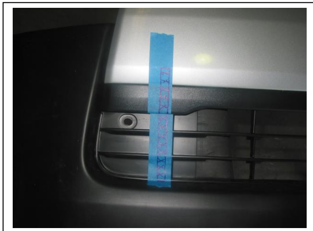
Figure 15 – Area that needs to be cut to fit over steel mount.
