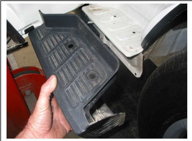
Figure 1 – Shown removing passenger side step infill
