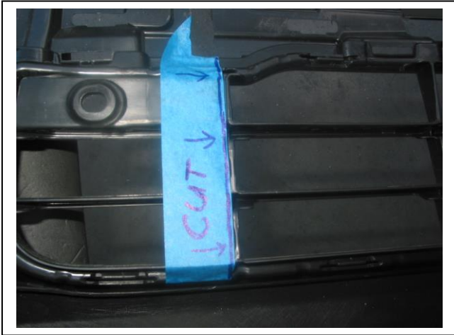
Figure 13 – Cut end off grille.
